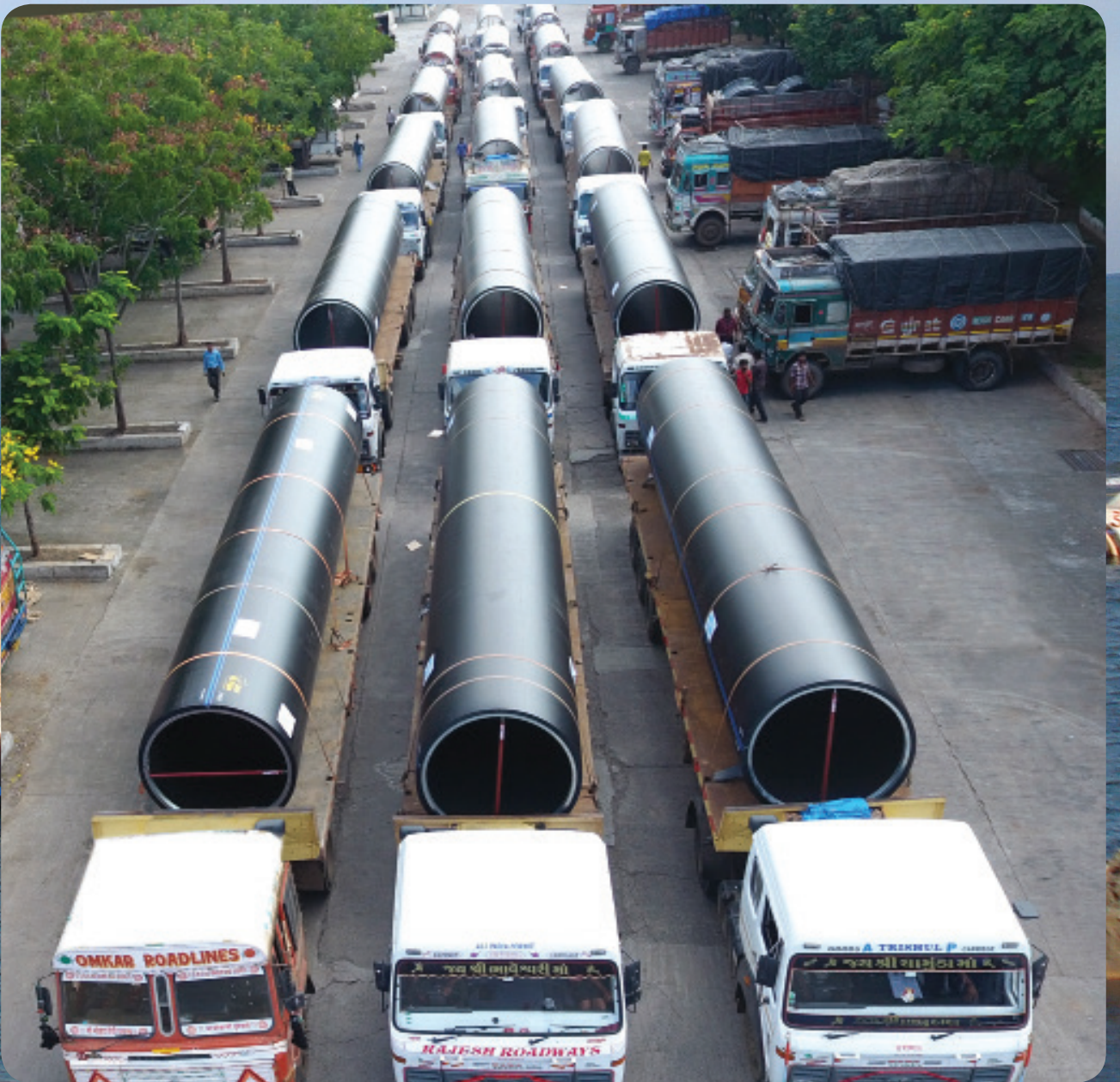
2000mm HDPE Pipes ready for despatches
